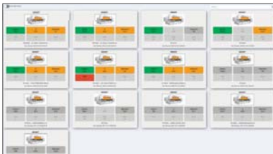
■ ACTIVE MACHINE CONTROL SCREEN It allows to monitor all machines operating in the field on a single screen for the error, warning, efficiency data.
