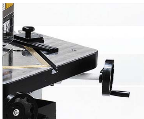
■ Hand wheel to help determining corner angle
