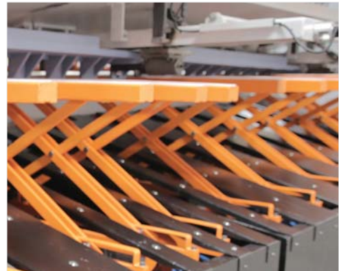
■ X type sheet metal support system operates parallel to ground to support the sheet metal during cutting period (O)
