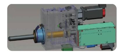
Precision Gear Transmission Headstock
