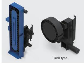
Neway's mechanical cam type tool change mechanism offers servo drive and allows a fast, reliable tool change for lower cycle times when several tools are required.
