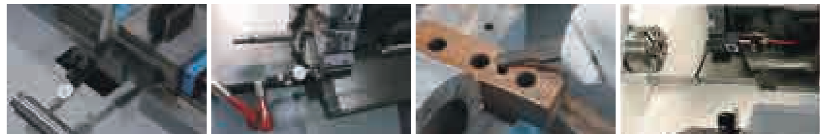
• Assembly inspection • Boring bar concentricity inspection • Hand scraping • Laser calibration
