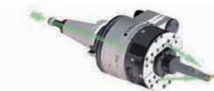
The coolant is ejected from the two adjustable nozzles on the side of the face plate through the taper shank and the facing head rotating body. This significant advantage extends tool life, increases cutting speed and guarantees surface finish quality.
