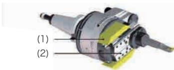
Face plate is equipped with two counter weights, which are automatically balanced by an opposite movement of the slide, thus enabling supported high-speed machining without significant vibration.
