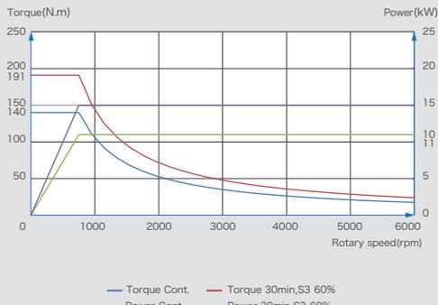
High torque spindle T-n, P-n diagram
