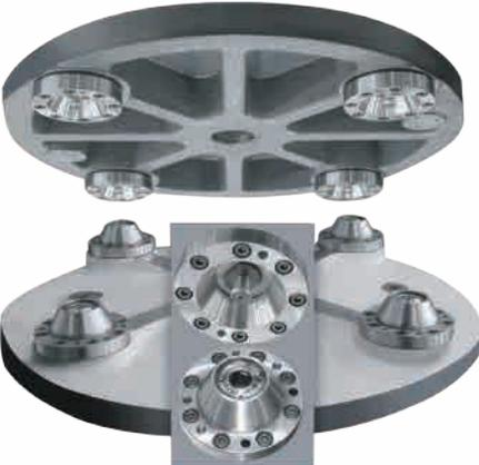
The pallet positioning adopts four-point cone positioning, which is excellent in rigidity, ensuring accurate positioning during work. When the table is exchanged, the four cones on the table blow out compressed air to prevent chips from entering.
