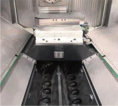
Iron scraps on both sides of the table are pushed directly into the rear sewage lifting system by a set of spiral chip eliminators. Achieve fast and efficient back chip remove. The front and rear screw row is arranged in an inclined manner, which can discharge chips more smoothly.
