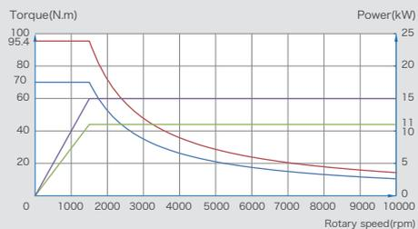
BT50 High-speed spindle T-n, P-n diagram
