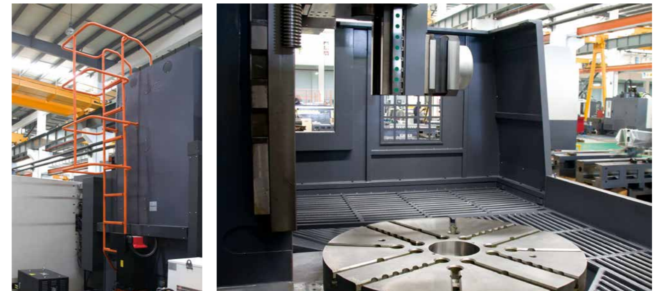
Ladder fence with a wide inside space is easy and safe for up and down. wide internal space and sliding door easy for the workpieces' loading and unloading.
