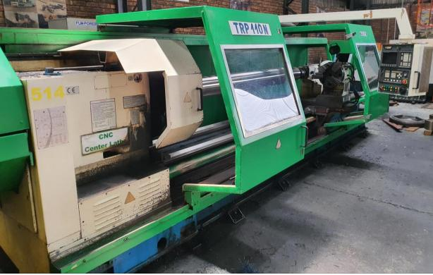
The POREBA CNC lathe Model TRP110N is designed for efficient and precise machining of large-size shafts. Thanks to the innovative mechanical solutions and advanced control systems, the multipurpose lathes ensure productive rough and finish machining. The TRP Series lathes are designed for workpiece machining in the range of turning in accordance with their specifications. It can operate as a horizontal machining center with capabilities for turning, drilling, and milling.
