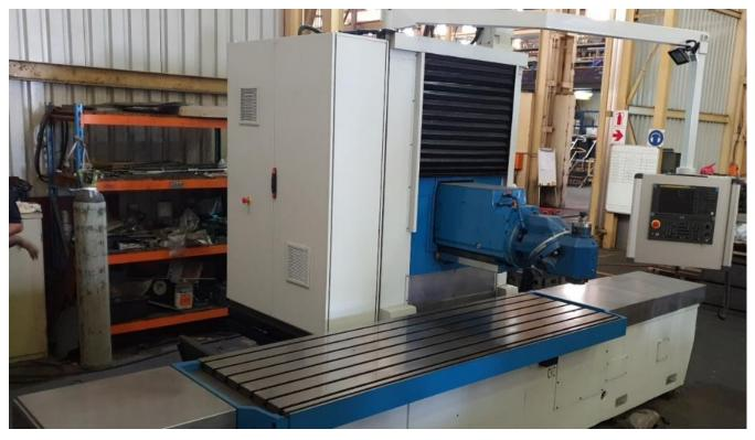
The Nicolas Correa A20-25, a CNC bed-type milling machine known for its robust construction and capability for heavy-duty machining, is part of Nicolás Correa's esteemed lineup of milling machines, recognized for their reliability and precision. With a generous table size and extensive travel on all axes, the A20-25 model is well-equipped to handle large workpieces.
